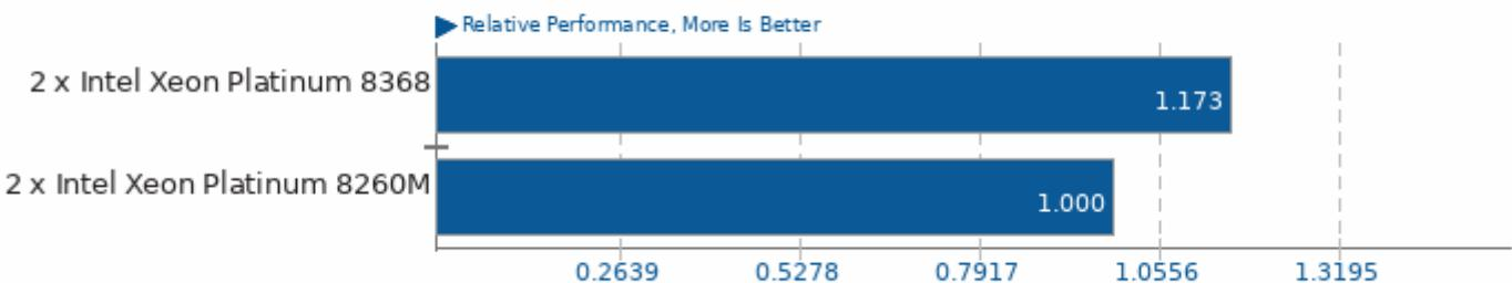
Geometric mean based upon tests: pts/apache, pts/nginx, pts/mysqlslap, pts/pgbench, pts/redis, pts/cassandra, pts/phpbench, pts/openssl and pts/sqlite-speedtest
