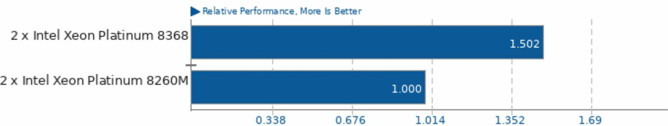
Geometric mean based upon tests: pts/lammps, pts/npb, pts/dolfin, pts/neat and pts/qe
