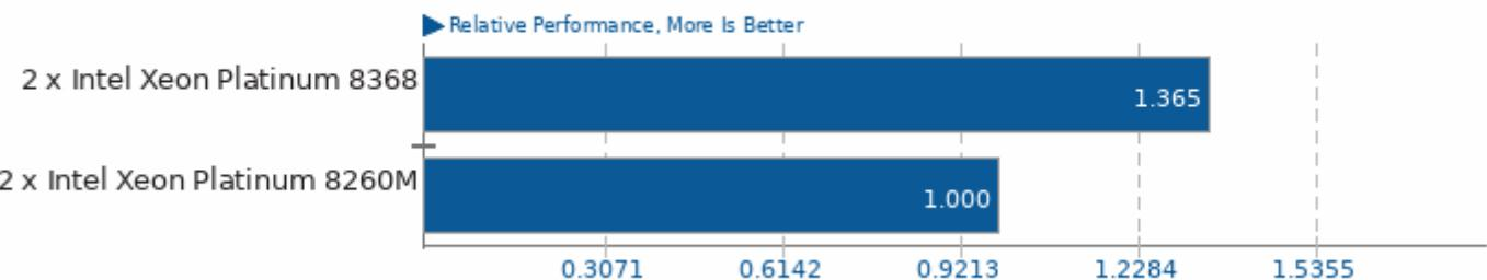
Geometric mean based upon tests: pts/build-linux-kernel, pts/build-gcc and pts/build-llvm
