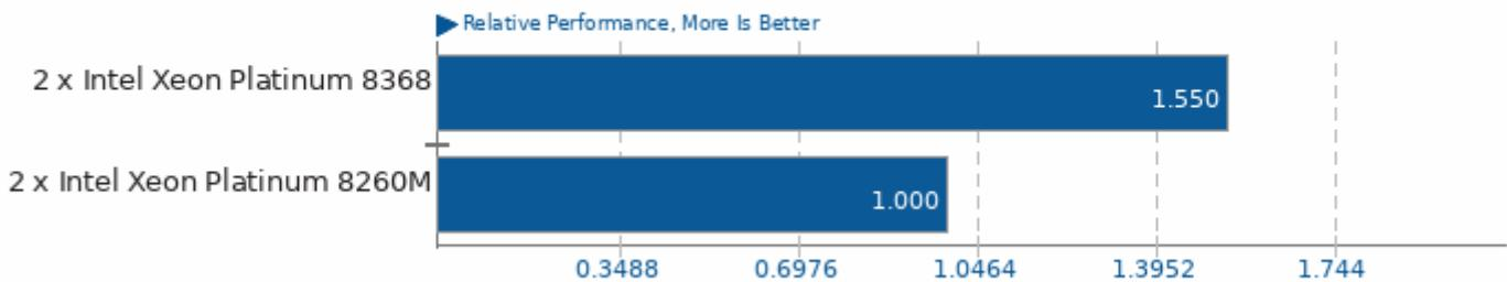
Geometric mean based upon tests: pts/blender, pts/rodinia, pts/himeno, pts/x265 and pts/sysbench
