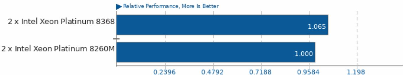
Geometric mean based upon tests: pts/java-scimark2, pts/byte, pts/cachebench, pts(numpy, pts/compress-gzip, pts/encode-flac, pts/encode-mp3, pts/gnupg, pts/redis, pts/pybench, pts/phpbench and pts/nginx
