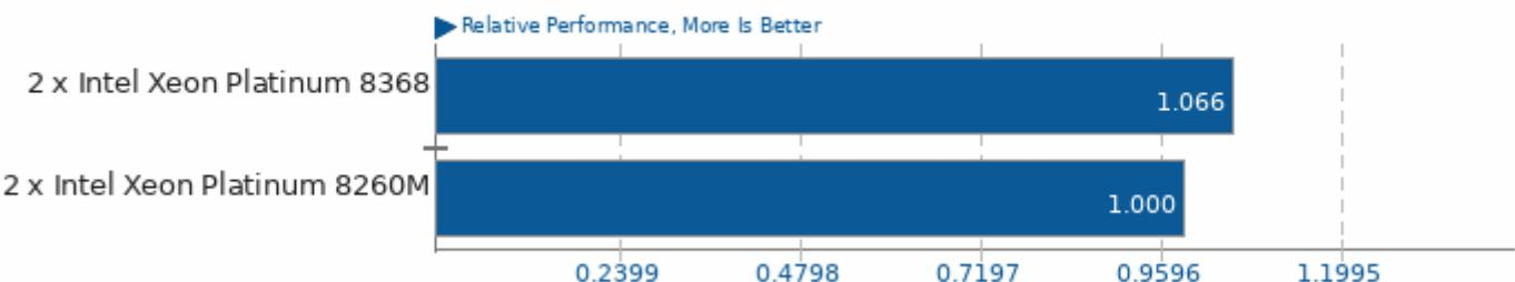
Geometric mean based upon tests: pts/pybench, pts/numpy and pts/pyperformance
